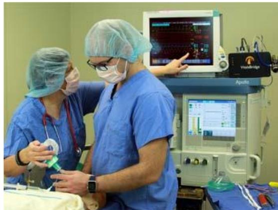
Vitals signs can be easily controlled from the VitalsBridge Connector Software or mobile app. The VitalsBridge can also be connected to your patient simulator software allowing for vital sign changes made in the software to seamlessly update on your patient monitor.
