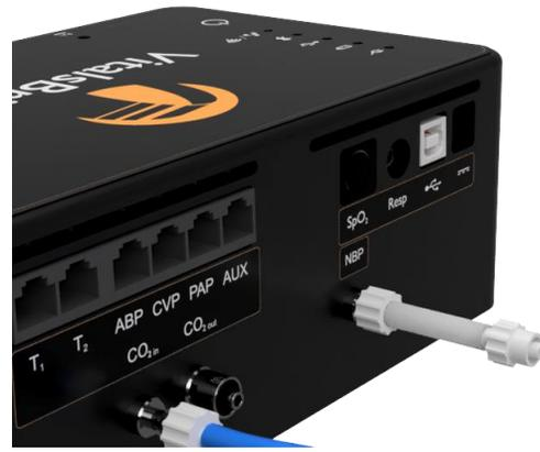
Affix the tube and luer fittings to each other to provide an ending that can be attached to the monitor NIBP tubing
