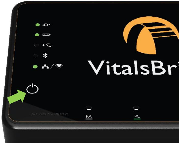
Check the status indicator lights on top of the VitalsBridge instrumentation to determine power and connectivity.
