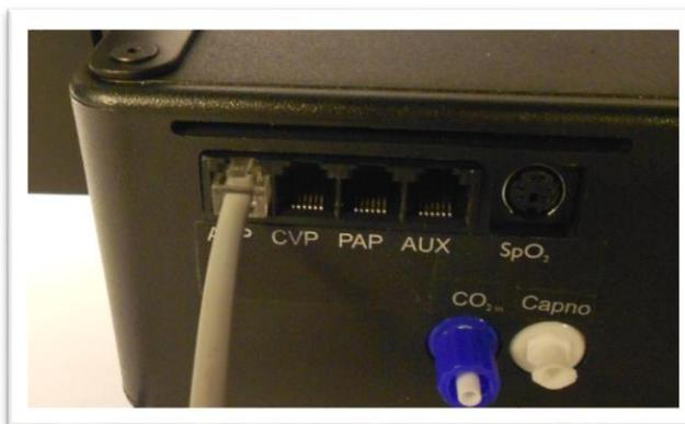
When using IBP, all waveforms are not required to for the VitalsBridge to function. Unused IBP ports on the VitalsBridge may be left unconnected.
