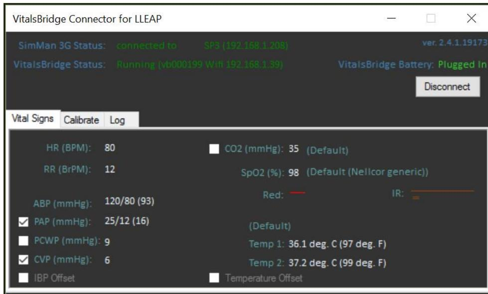
The VitalsBridge software allows the user to monitor connectivity between the VitalsBridge and the patient simulator, calibration of SpO<sub>2</sub>, CO<sub>2</sub>, temperature signals, and configuration of a few additional settings.
